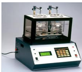
Disintegration test apparatus
